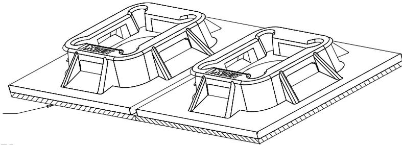
ADHESIVE BACKING: (-A, -AT) RUBBER OR ACRYLIC BASED ADHESIVE PRESSURE SENSITIVE FOAM TAPE 0.04 [1.0] THICK WITH A PROTECTIVE LINER. MOUNT IS DESIGNED TO SUPPORT 0.50 lbs (227g) MAX. WEIGHT ON A CLEAN DRY SMOOTH SURFACE.
