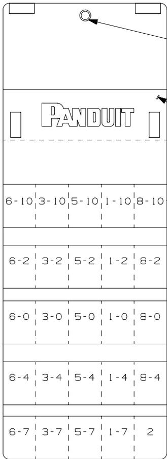
EYELET FOR SUSPENSION FROM NAIL, SCREW OR CABLE TIE.
