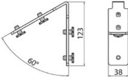
The element is ready for composition at fixed degree but it is a sliding system inside the section itself (1). The possibility of tightening using an Allen spanner (2) significantly speeds up assembly and neither bolts nor nuts, nor various locking system protrude from the sections themselves (3). This provides a continuous base without rough spots or elements outside the profiles (4).
