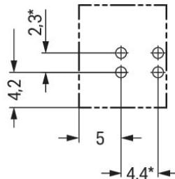
Drilled hole diameter:  $1.3^{+0.1} \text{ mm}$
