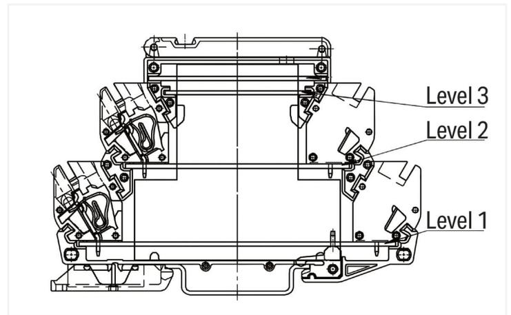
Universal modular component plug housing, as rail-mount terminal block – transparent cover
