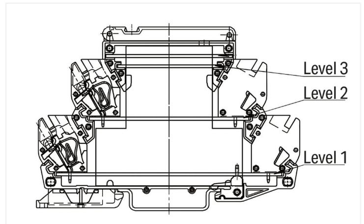
Universal modular component plug housing as rail-mount terminal block – 55 mm cover
