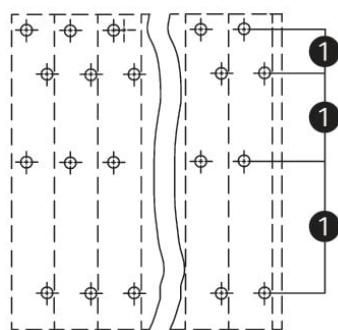
(1) Solder pins for deck 2 and 4 staggered by half the pin spacing
