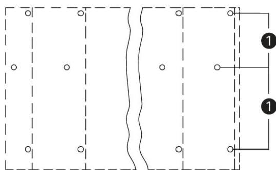
(1) Solder pins for deck 2 staggered by half the pin spacing
