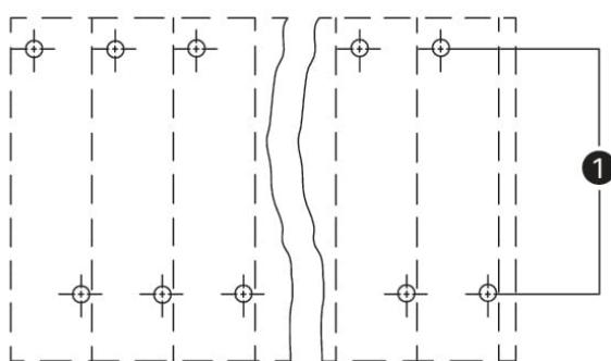
(1) Solder pins staggered by half the pin spacing
