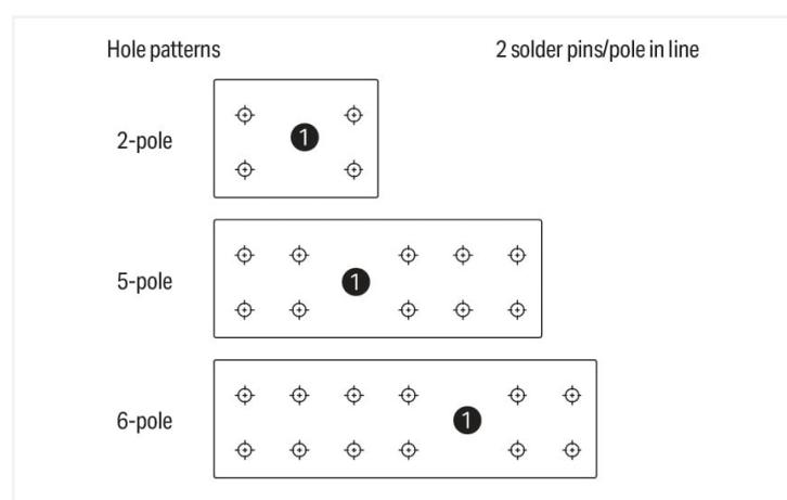
(1) Spacer: 1 x pin spacing
