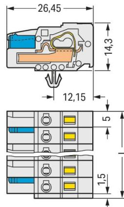
Side view dimensions: total width 26.45, height 14.3, depth 12.15, and overall length L.
