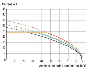
2-, 4-, 6-, 12-pole      Conductor rated current
