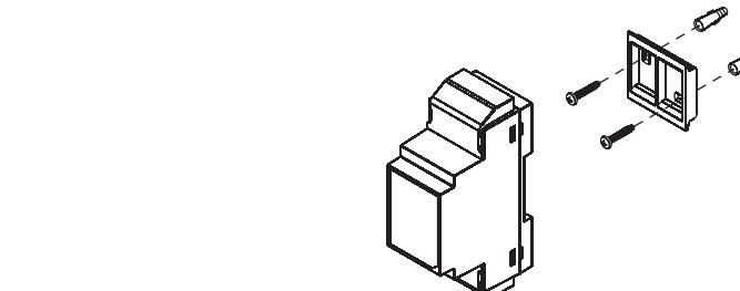
In case of wall mounting, a terminal pin protection cover MUST be installed.
