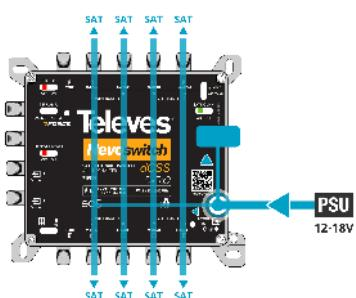
Switches: TERR.DC - ON, RECEIVER POWER – OFF, SAT DC LINK – ON
