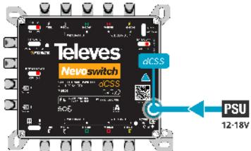
Switches: TERR.DC - OFF, RECEIVER POWER – OFF, SAT DC LINK – ON
