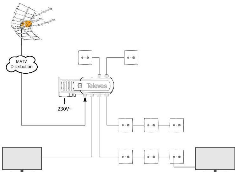
Connector type and number of outputs according to reference
