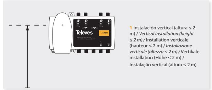
1 Instalación vertical (altura ≤ 2 m) / Vertical installation (height ≤ 2 m) / Installation verticale (hauteur ≤ 2 m) / Installazione verticale (altezza ≤ 2 m) / Vertikale installation (Höhe ≤ 2 m) / Instalação vertical (altura ≤ 2 m).
