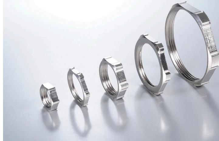
To ensure permanent bonding between the cable gland and housing in painted or coated housings, a lock nut with 6 teeth which cut into the coating automatically when tightened, thus providing equipotential bonding. Moreover, this type of attachment increases the installation's resistance to vibration.
