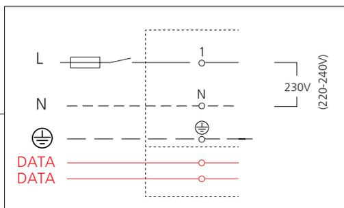
• Standard DALI control gears are only to be used if they fulfill the **SELV** ( Safety-Extra-Low-Voltage) requirements or use **SELV** safety pcb.
