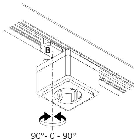
Turn knob **B** 90° clockwise to connect the adaptor to circuit **1**.
