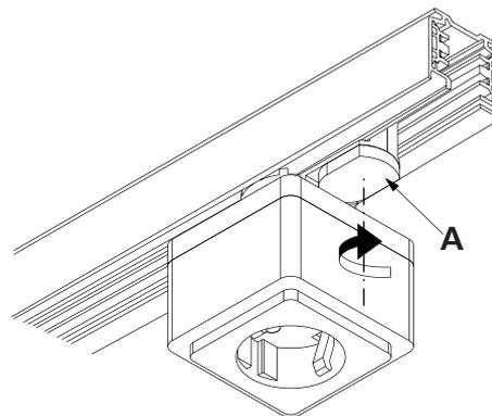
Turn knob **A** 90° clockwise to connect the adaptor to the neutral circuit **0**.
