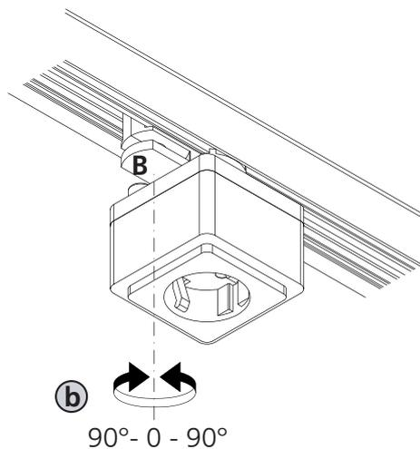
Pull knob **B** out and turn 90° anti-clockwise to connect the adaptor to circuit **3**.
