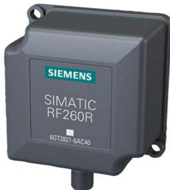
SIMATIC RF200 Reader RF260R interfaccia IO-Link V1.1; IP67, -25 ... +70 °C; 75x 75x 40 mm; con antenna integrata 32 byte IO; 230 kBit/s.
