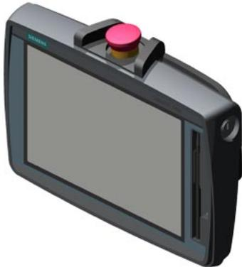
SIMATIC HMI TP1000F MOBILE 10.0" TFT display, 1280x800 pixels, 16 million colors, Touch operation, touch pen, 1x PROFINET/Industrial Ethernet interface, 1x multimedia card, 1x USB, key-operated switch, acknowledgement button, 1 emergency stop/stop button configurable from WinCC Comfort V14
