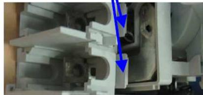
Remove the internal sub assembly from the base and cut the electrical wires to remove the printed circuit boards from the sub assembly
