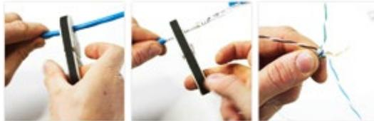
Use the cable stripper tool and cut the outer sheath.
