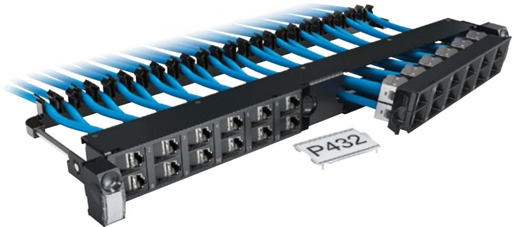
The flat data panel contain a configuration for 24 RJ45 connectors with a clear marking at both front and rear. The panels are easy to install thanks to the front access and the Quick Fix function. Use the vertical side rings for vertical management of the patch cords. Other features are the removable cable manager at the rear, the panel identification label and the hinged central label holder.
