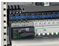
Linerage FM device feeder 80 A. The Linerage FM device feeder snaps easily onto the back of the rails. All types of modular devices can be mixed in the same row and phase balancing is simple. It's easy to change or add devices.
