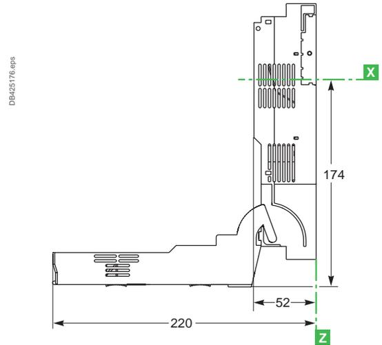
Device to be installed on a busbar
