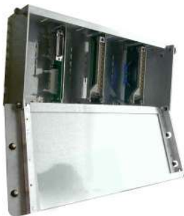
Chassis for Modicon Premium PLC modernization
