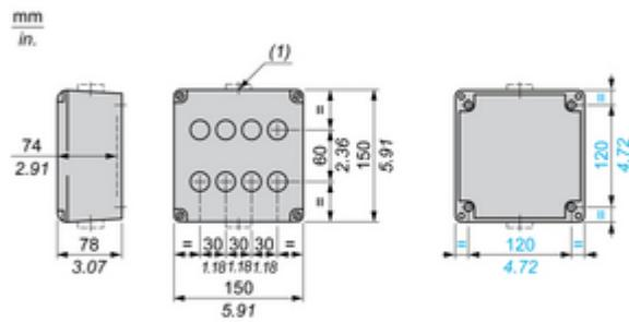
(1) 2 holes (with plug, 7.5 mm / 0.29 in. protrusion) for cable gland, max clamp Ø12 mm / 0.47 in.
