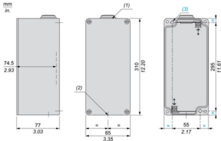
(1) 1 hole (with plug, 6 mm / 0.24 in. protrusion), for cable gland ISO M32 x 1.5
