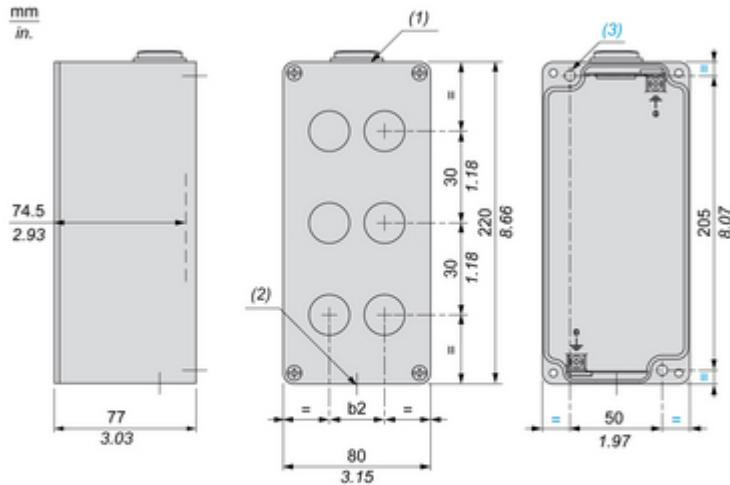
(1) 1 hole (with plug, 6 mm / 0.24 in. protrusion), for cable gland ISO M25 x 1.5
