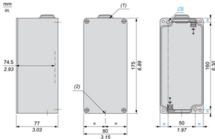
(1) 1 hole (with plug, 6 mm / 0.24 in. protrusion), for cable gland ISO M25 x 1.5
