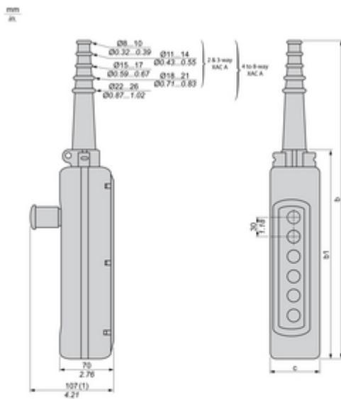
(1) With trigger action Emergency stop head operator
