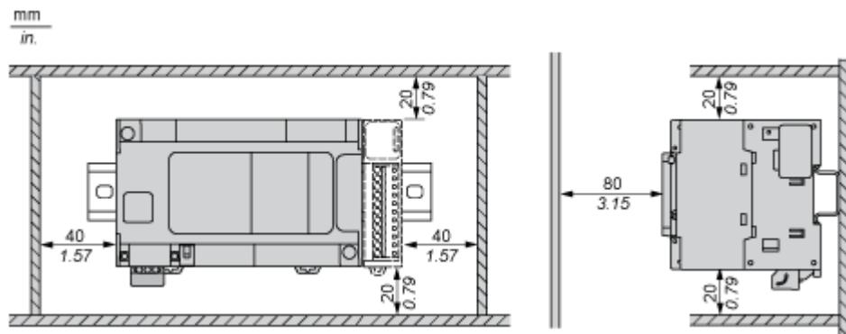
**Posizione di montaggio**
