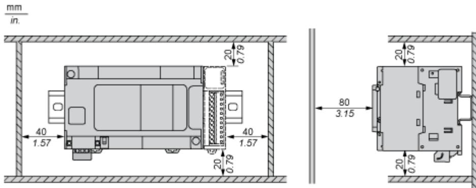
**Posizione di montaggio**
