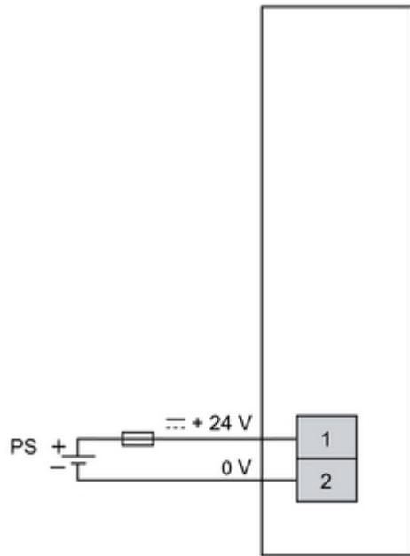
PS : External isolated power supply, 24 Vdc
