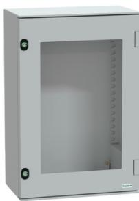
Cassetta in poliestere montata a parete, PanelSeT PLM, porta trasparente, 647x436x250mm, IP66, IK08, RAL 7035
