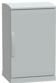
Armadio in poliestere, PanelSeT PLA, fondo aperto, tetto ventilato, 750x500x420 mm, IP44, IK10
