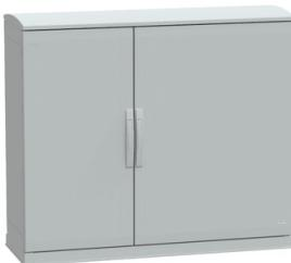
Armadio in poliestere, PanelSeT PLA, fondo aperto, tetto ventilato, 1000x1250x420 mm, IP44, IK10
