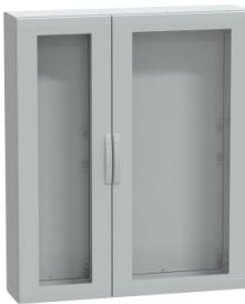
Armadio in poliestere, PanelSeT PLA, porta trasparente, totalmente chiuso, 1500x1250x320mm, IP65, IK08
