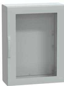
Armadio in poliestere, PanelSeT PLA, porta trasparente, totalmente chiuso, 1000x750x320mm, IP65, IK08
