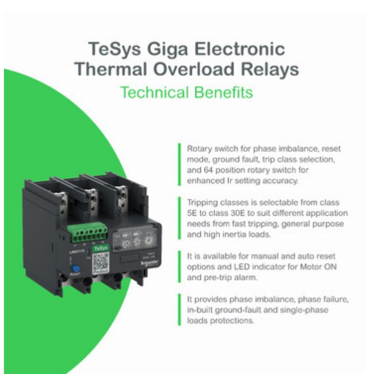
**TeSys Giga Electronic Thermal Overload Relays**
