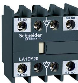
Auxiliary contact block, TeSys Deca, 2NO(sealed)+2NO, front mounting, screw clamp terminals
