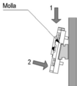
**Montaggio e fissaggio del rack sui pannelli**
