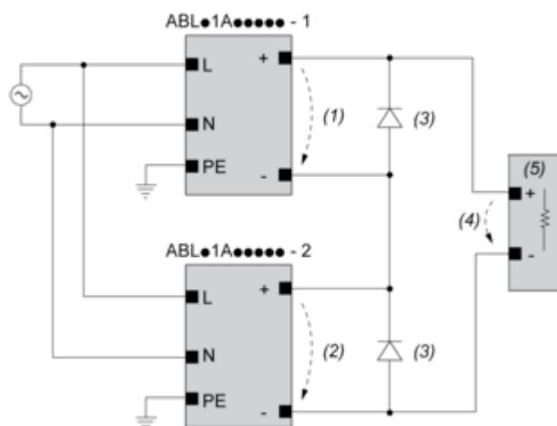
(1):  $V_{out1}$ (2):  $V_{out2}$ (3): 2 diodi,  $V_{RRM} > 2 \times V_{out1/2}$ ,  $I_F > 2 \times I_{nom1/2}$ (4):  $V_{Load} = 2 \times V_{out}$
