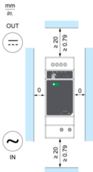
**Posizione di montaggio A**
