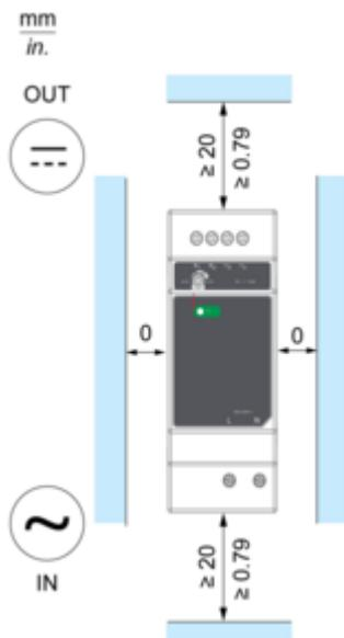
**Posizione di montaggio A**
