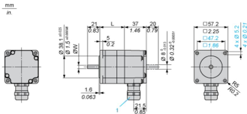
1: Passacavo M20 x 1, per cavo  $\varnothing 9 \dots 13$  mm / 0.35 ... 0.51 in.
