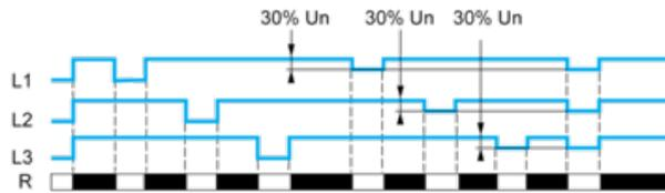
Control of Overvoltage and Undervoltage
