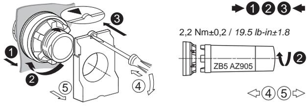
For use on flat surface of a type 4, type 4X, type 12, and type 13
