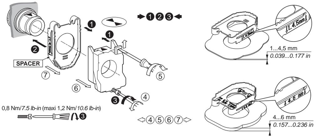
For use on flat surface of a type 4, type 4X, type 12, and type 13
