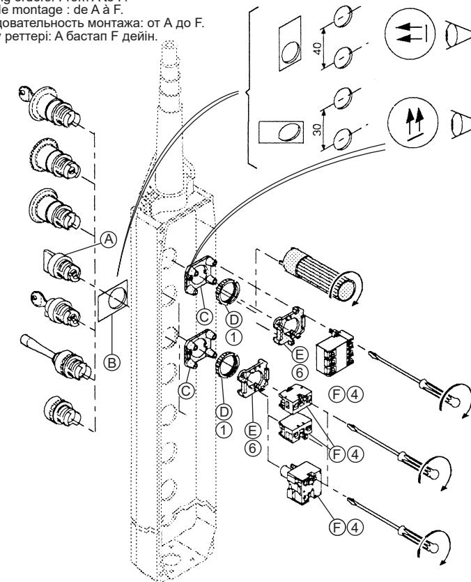
Mounting with components ZA2 B in base of enclosure
