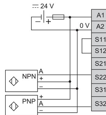
**NOTE:** The sensors must be supplied by the same PELV/SELV power supply as the safety module.
