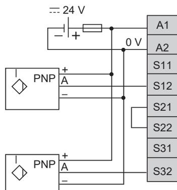
Proximity detectors with NPN and PNP outputs - With detection of short circuits
